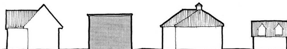
Flat roof incompatible with nearby gables and hip roofs
